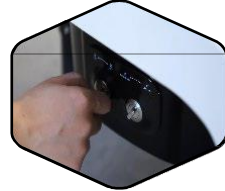
Disconnect the power Prevent damage to the work caused by touching the foot pedal by mistake when picking up the work
